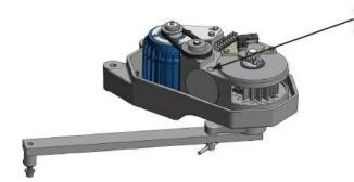
Remove the cover to lubricate the worm screws
